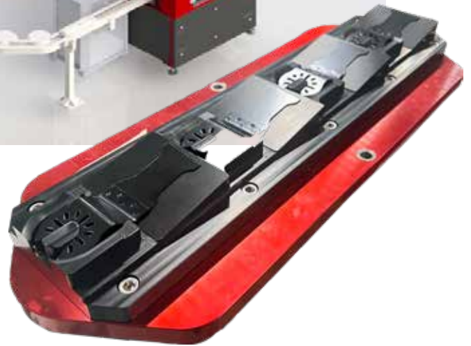
Spider robot loads the fixture above, which moves continuously around the racetrack conveyor.
